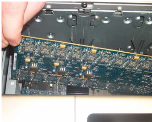
Figure 3. Sliding the front of the card into PCIe card support
